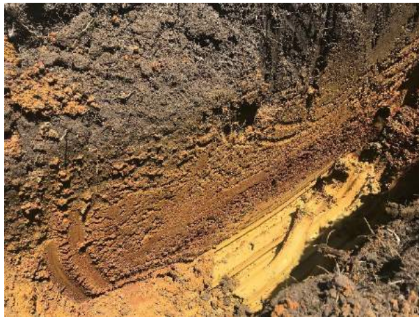
TP211 – Mottled orange alluvial clay (Unit 4) overlying residual (Unit 5) yellow clay.
