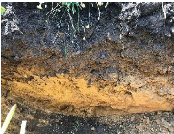
TP208– Colluvial gravelly clays to 0.5m where moisture can concentrate, overlying residual low CBR yellow clay (Unit 5) grading into highly weathered dolerite from 0.9m
