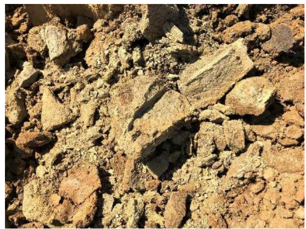
TP203 – Highly weathered dolerite (Unit 7) present from 1.1m below the surface and excavated as low strength gravel.
